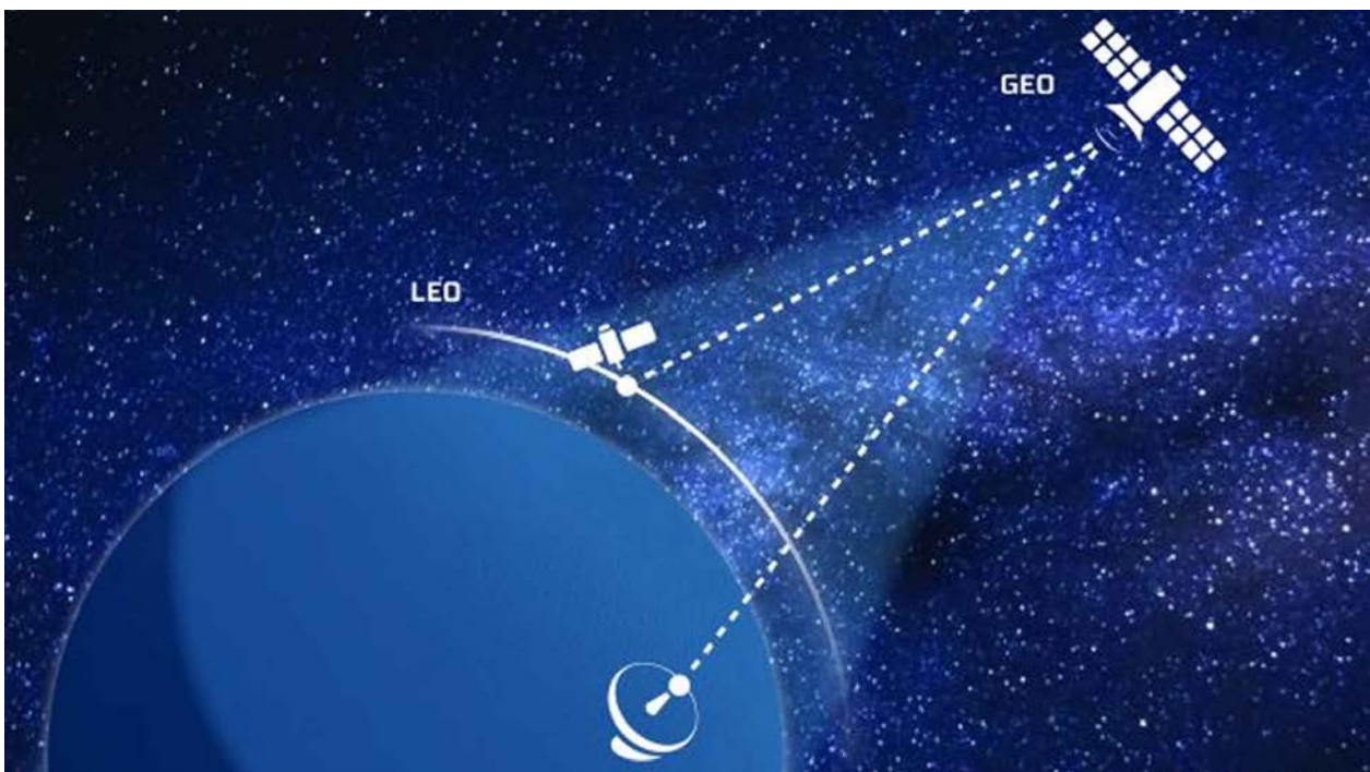
Illustration of how IDRS connects LEO satellites to the ground via GEO satellites.
