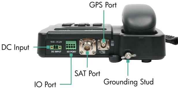
**DC Input:** Power input connector is used for connecting the external power source (10.8 ~ 31.2 volts) to the Base Terminal
