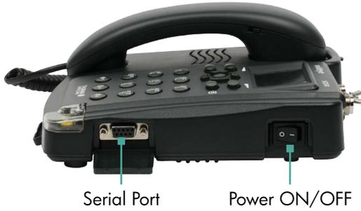
**Serial Port:** This is a 3 wires (TX, RX and ground) RS232 port. It is for Terminal Firmware upgrade.
