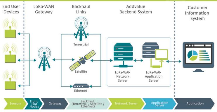
Addvalue LoRa-WAN solution provides key building blocks from customer's end user devices to customer information system, enabling diverse applications in various different vertical markets.
